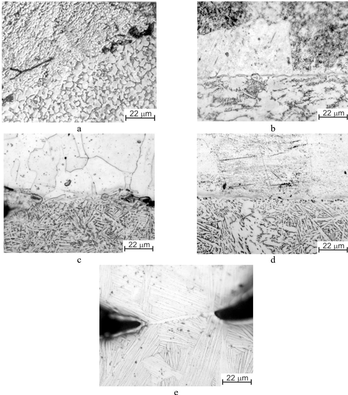
**Fig. 5.** Microstructure of the base-coating interface obtained by plasma spraying (a, c), 3D-printing (b, d), using POROCOAT® and GRIBTION® technologies (e). After annealing (a, b, e) and thermal hydrogen treatment (c, d)
