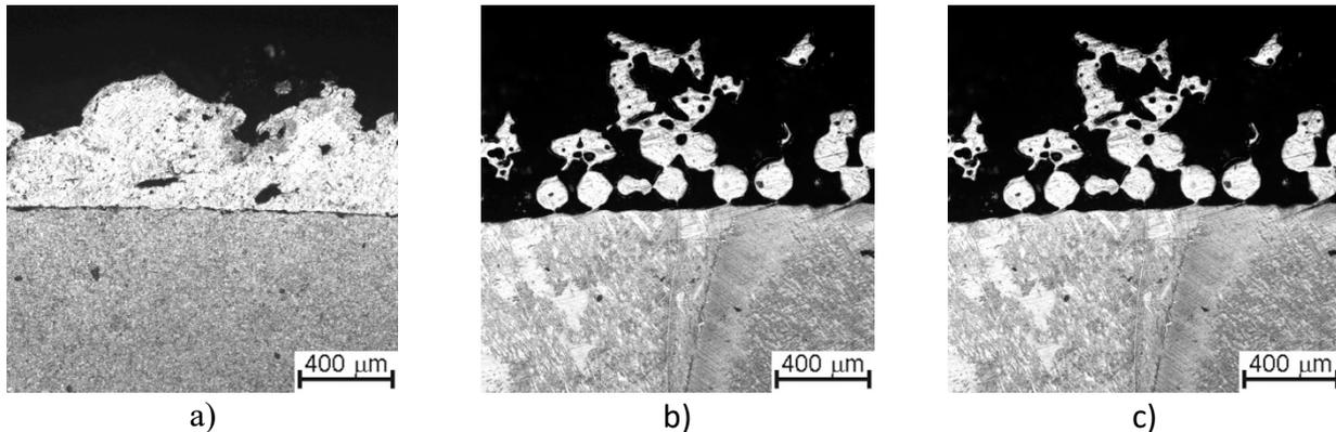
**Fig. 2.** Structure of porous coatings obtained by plasma spraying (a), using GRIPTION® technology (b), and DLMD (c)
