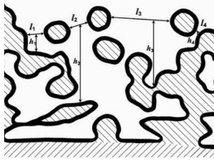
Fig. 3. Scheme for measuring pore width and depth.
