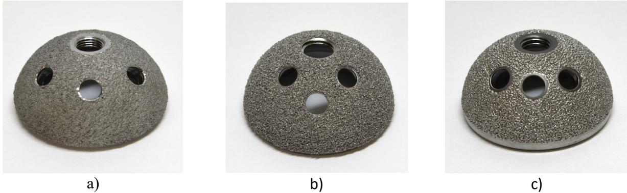
**Fig. 1.** Appearance of bowls obtained by plasma spraying (a) using GRIPTION® technology (b) and DLMD (c)
